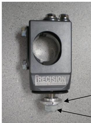
If holes in stock steering stems top plate are less than 10mm you will need to drill at least 2 holes to 10mm.
