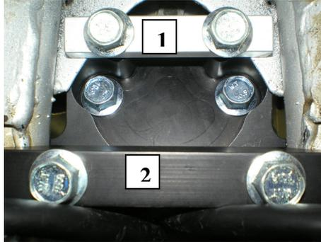
The stabilizer mounts in front of the steering stem and on the chassis where the upper A-arms attach.
