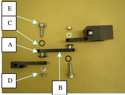
Re-grease the linkage every 20 hours, more often if pressure washing the quad. Remove linkage bolts, clean and re-grease link-arm and bushings. Re-assemble then torque screws to 9 ft-lb.
