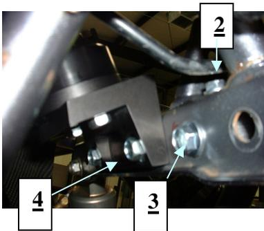
Attach the stem clamp to the stem snug the 6mm screws
