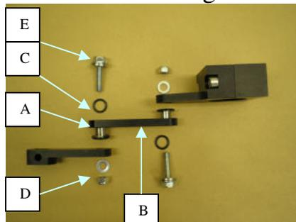
Re-grease the linkage every 20 hours, more often if pressure washing the quad. Remove linkage bolts, clean and re-grease link-arm and bushings. Re-assemble then torque screws to 9 ft-lb.
