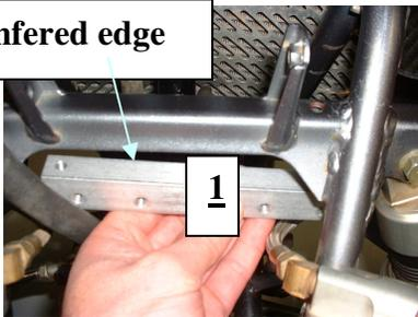
Install 6mm screws finger tight into 2
