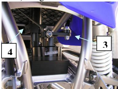
Insure screws are tight and aligned and that there is no interference with brake lines or other components when the bars are rotated.
