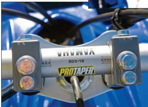
used to adjust the tension of the clamps. Adding more shims removes flex, and vice-versa.
